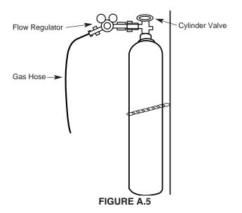
Attach the flow regulator to the cylinder valve and tighten the union nut securely with a wrench.
